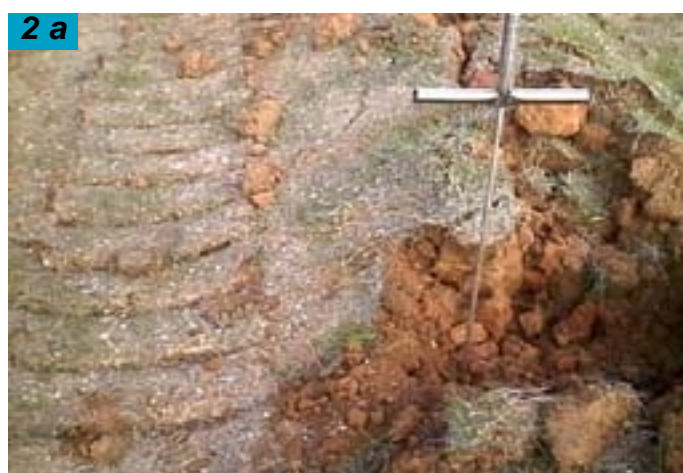
Fig 2. Measuring soil penetration resistance
