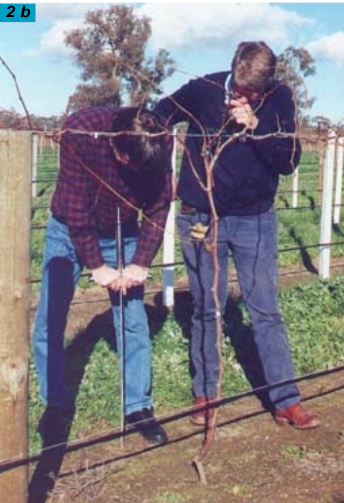
Fig 2. Testing soil penetration resistance. a) during deep ripping to ensure a good result b) after a season to check for tractor compaction.
